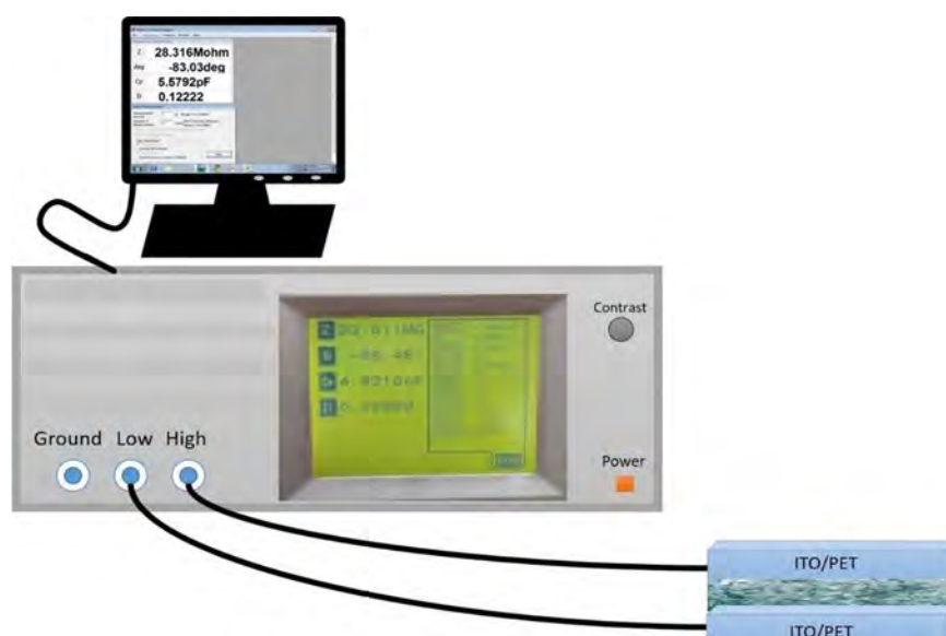
Figure 3. Schematic diagram of the experimental setup for measuring the relative change in capacitance concerning different applied pressures for the fabricated device (as shown in Figure 1).
